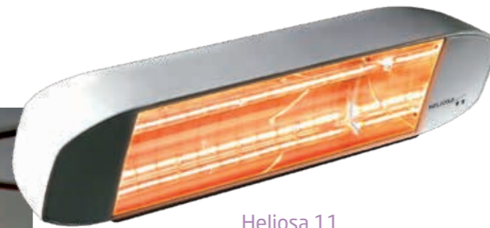
Heliosa 11 2000 W, IP20 (11B20) Installation height 1,90-2,20 m Heating surface 12-15 m 2 Dimensions 45,5x13x9 cm
